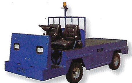
Maintenance Cart 48 Volt System
